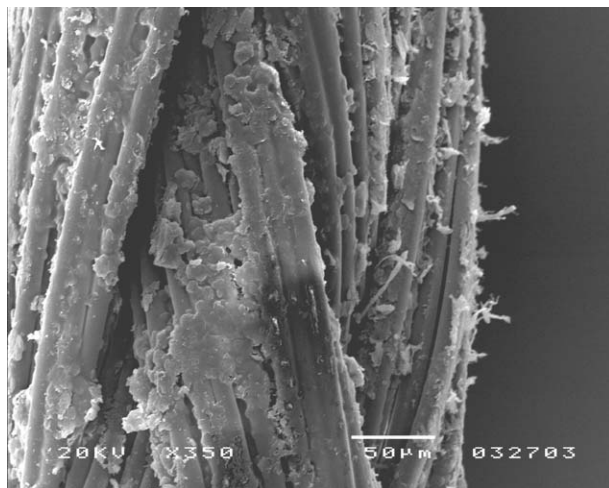
Figure 1 SEM micrograph showing the as-received Vicryl ® suture.
